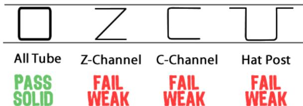
The Benefits of the Tube Frame Outweigh Any Slight Cost Difference! The Tube Frame Eliminates the Twisting and Vibration Found in the Typical Cargo Trailer and Gives You a Smoother Pulling Trailer.
