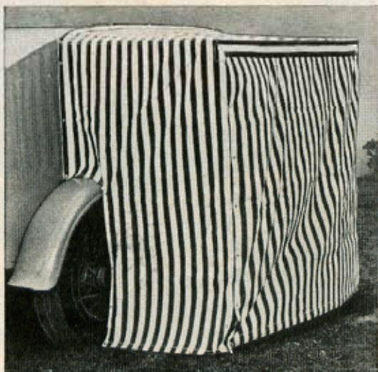
AS A DRESSING ROOM, the cabana provides an area 3 ft. deep and nearly 5 ft. high and wide. The camper's threshold makes a handy seat. The rear of the fabric is snapped to the camper body all around
