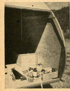
Photo 1. Showing rear end segments glued and screwed to sidewall. Also note splice batten and wheel house box.
