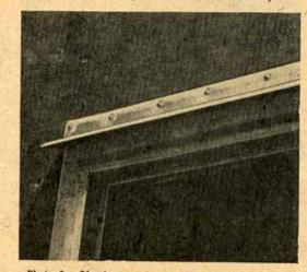
Photo 6. Aluminum strips are screwed around all raw edges of door, frame and body. Drip molding is bent and fastened above as shown.
