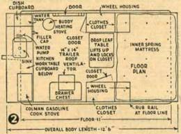
both sides, except the space where the wheels are. Now insert these fillers between frame ends and clamp with C-clamps. Drill a  $\frac{1}{4}$  inch hole down through each end of filler strip. Be sure to catch the frame wherever possible. These are then bolted with  $\frac{1}{4} \times 3$  inch carriage bolts all around both sides. Take light batten strips and screw underneath floor, crossways over the floor panel cracks, to keep out dust.
