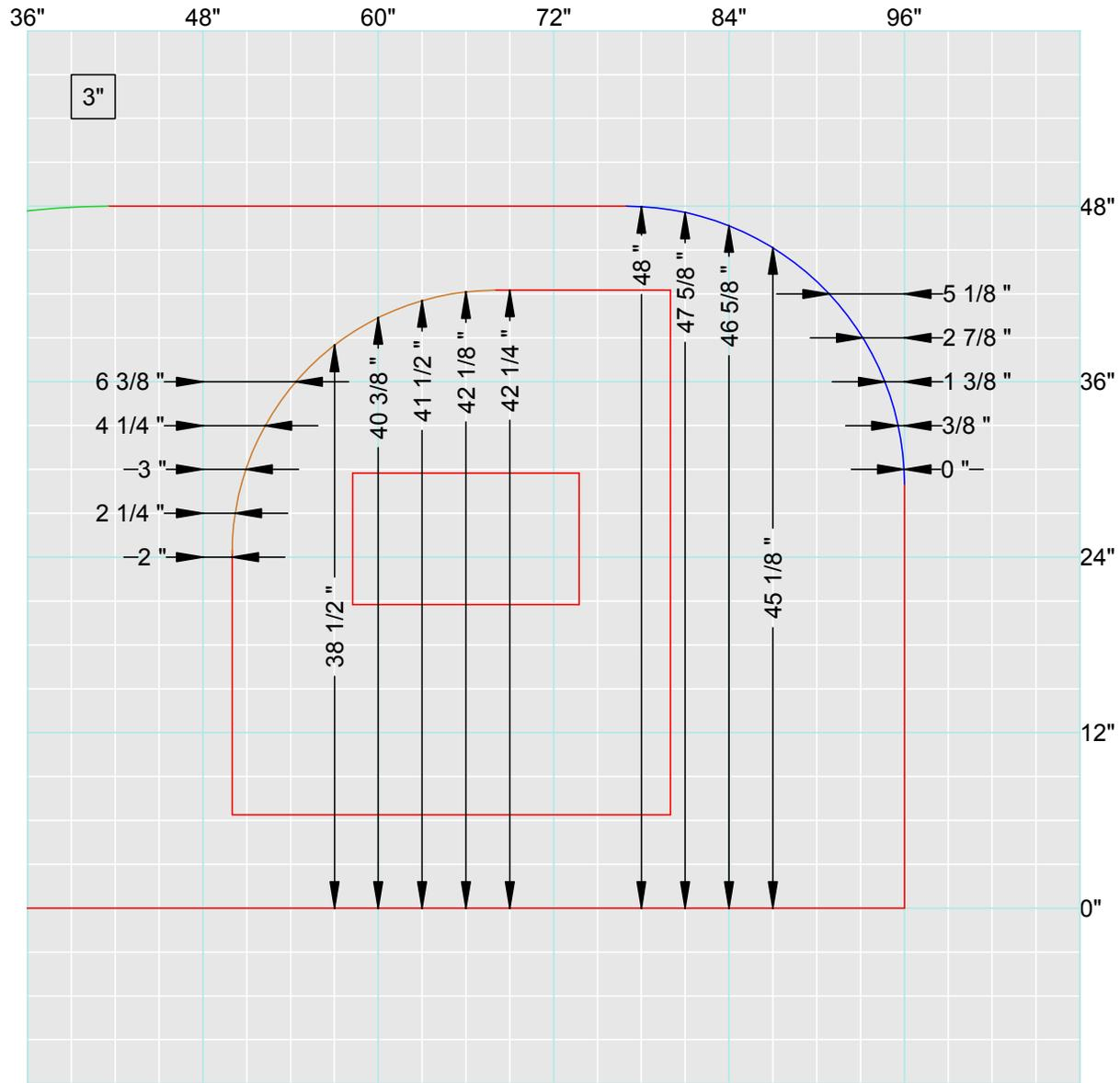
Note: It is recommended that these arcs are drawn using a compass (or string and nail), rather than by using the dimensions above.
