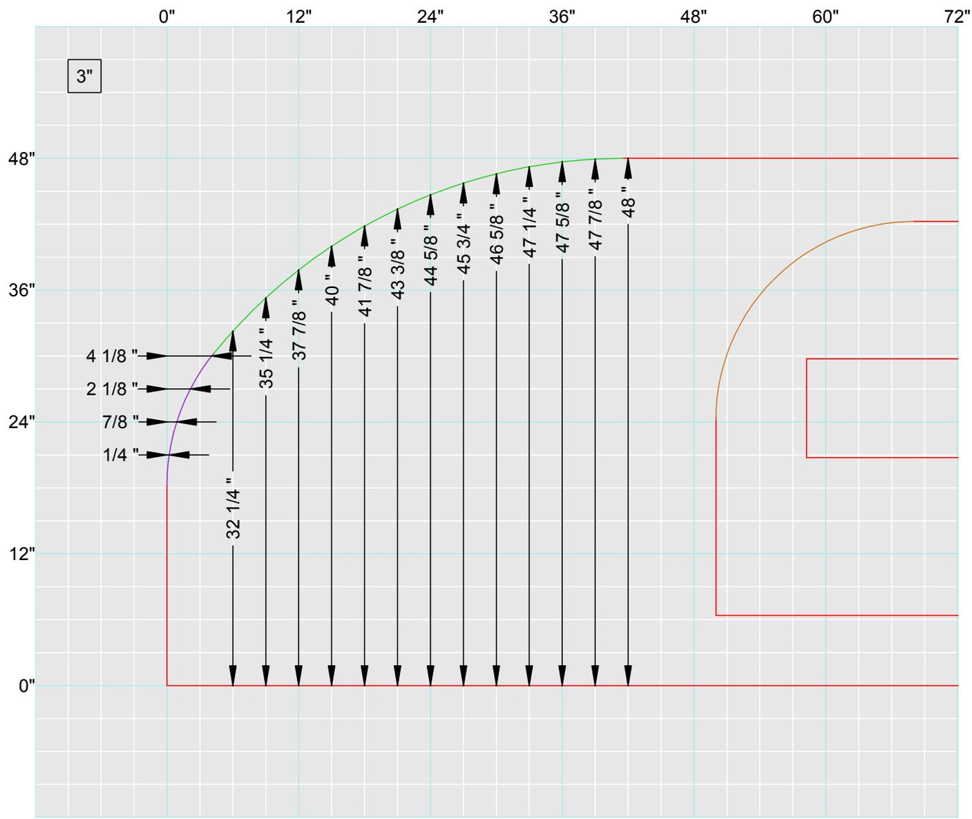
Note: It is recommended that these arcs are drawn using a compass (or string and nail), rather than by using the dimensions above.
